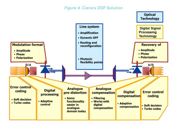
The physical optical equipment that provide the following functions are now performed in a single DSP ASIC (illustrated in *Figure 4* above).
