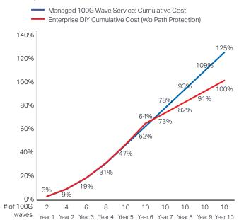
Analysis of enterprise annual costs (unprotected network): Analysis of enterprise implementing DIY in year 6 is to drop the annual OPEX by approximately 44 percent by year 7, thereby bending the enterprise cost curve as shown and leading to a 25 percent savings verses managed 100G waves service by year 10.
