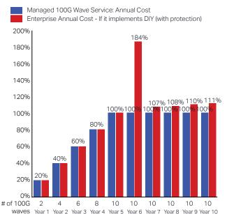
Analysis of enterprise annual costs (protected network): From year 1 to 5 enterprise paid OPEX for managed 100G wave service paid to CSP. Enterprise embarks on DIY in year 6, incurs a one-time CAPEX for terminals and two line systems and ongoing OPEX for terminals and two line systems and OPEX to CSP for two pair of DF lease/IRU and space/colocation and power
