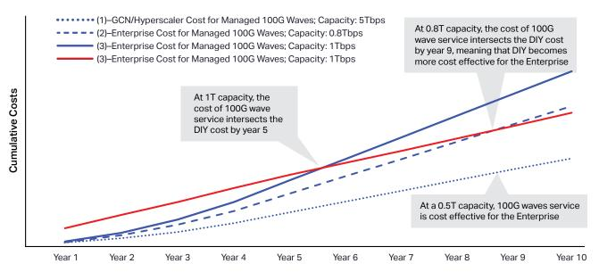
Figure 1. Enterprise cumulative costs for managed 100G wave service versus enterprise DIY for network capacity growth: 0.5T to 1T over 10 years
