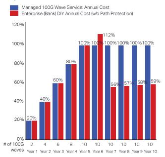
Analysis of enterprise annual costs (unprotected network): From year 1 to 5 enterprise paid OPEX for managed 100G wave service paid to CSP. Enterprise embarks on DIY in year 6, incurs a one-time CAPEX for terminals and line systems and ongoing OPEX for terminals and line systems and OPEX to CSP for DF lease/IRU and space/colocation and power.
