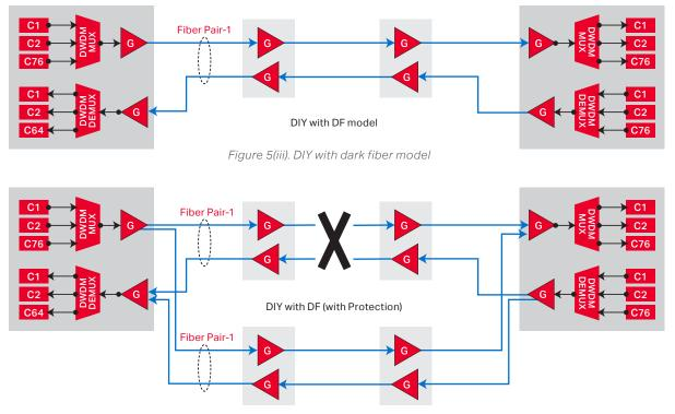
Figure 5(iv). DIY with DF model (with protection)
