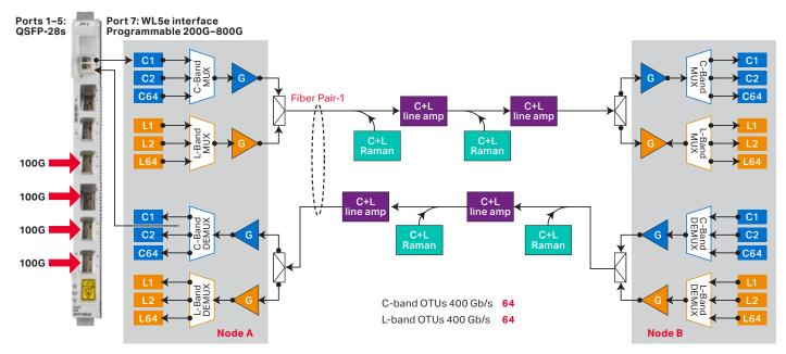
Figure 5(ii). Managed spectrum/wavelength service based on Ciena's integrated C&L-band architecture
